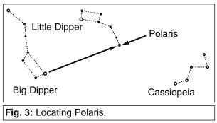
4. Without moving the telescope on the Right Ascension and Declination axes, loosen the azimuth and latitude locks (**9 and 30, Fig. 1**) and adjust the telescope until Polaris is centered in the telescope eyepiece. If steps 1 - 3 above were performed with reasonable accuracy, your telescope is now sufficiently well-aligned to the North Celestial Pole for visual observations.
